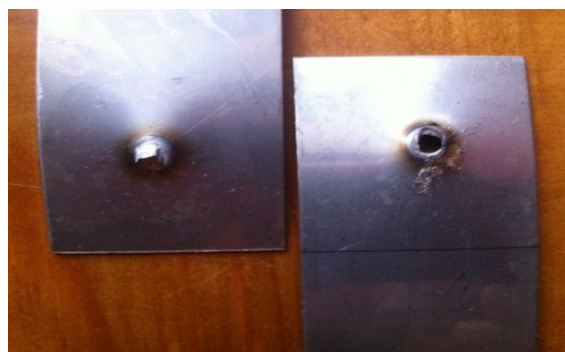
Figure 5 Failure mode in tensile test of AISI 304 resistance spot weld
